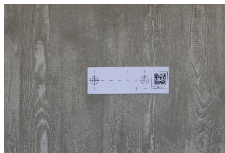
b) Example of marker with recommended size of 150mm (distance between targets)
